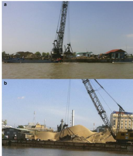
Photographs showing industrial-scale sand extraction operations in 2012 from the bed of the Bassac.
